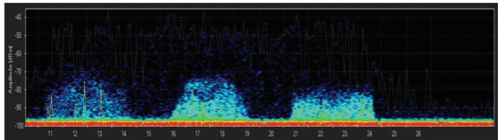
Figure 2: Hospital WiFi use of 2.4 GHz spectrum showing “gaps” at 802.15.4 channels 15 and 20
