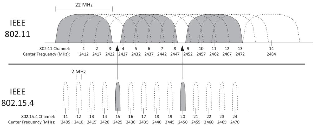
Figure 1: Use of the 2.4 GHz band by 802.11 and 802.15.4 systems
