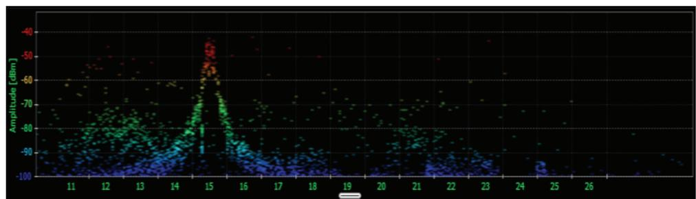
Figure 3: Leaf Patient Monitor use of 2.4 GHz on Channel 15
