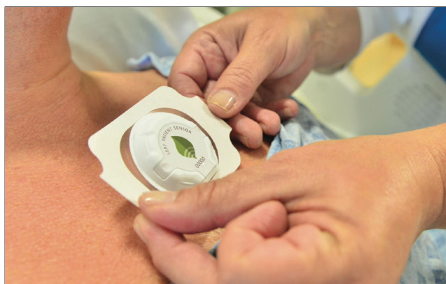
A sensor is applied to a patient's upper torso. The sensor continuously monitors the patient's movement and position. Sensor data is wirelessly communicated through a network of relay antennas and viewable on computer terminals or mobile devices.
