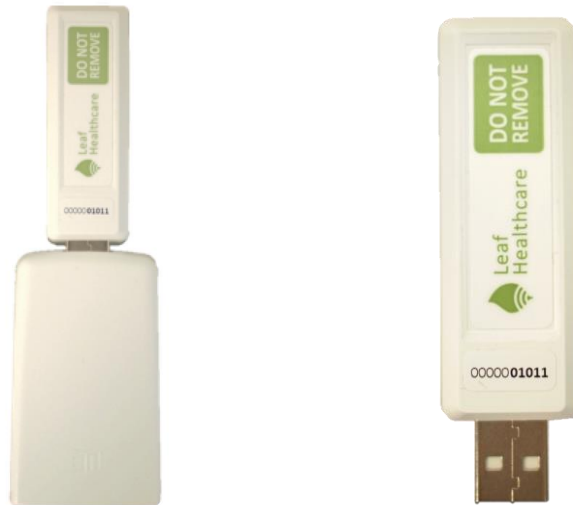
Figure 5: Leaf Antenna (Left) and USB RF Transceiver (Right)
